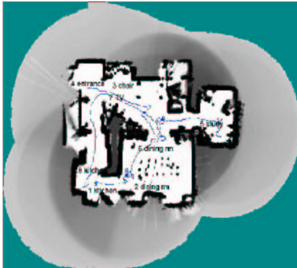
Figure 6.5: Laser range finding data from the ground floor of a house: Dark regions correspond to obstacles like walls and furniture, white regions correspond to free space. Once a map has been learned, any new obstacles which are not in the map are assumed to be people. In this way, the trajectory of a moving person (shown as a wiggly blue line) can be inferred. Various places where the person likes to spend a lot of time are labelled, and are considered landmarks or goals. This data is from [BBT02].
